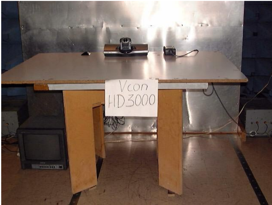
Figure 31. Conducted Emission Test
