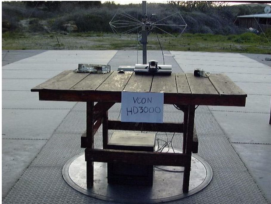
Figure 33. Radiated Emission Test
