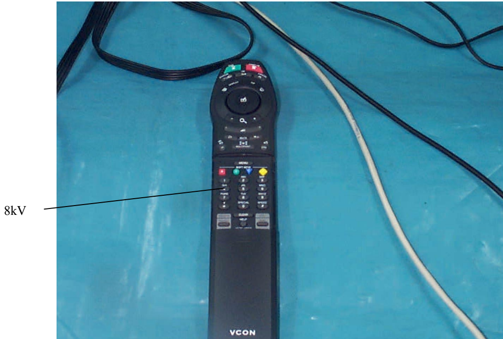
Figure 26. ESD Test Points
