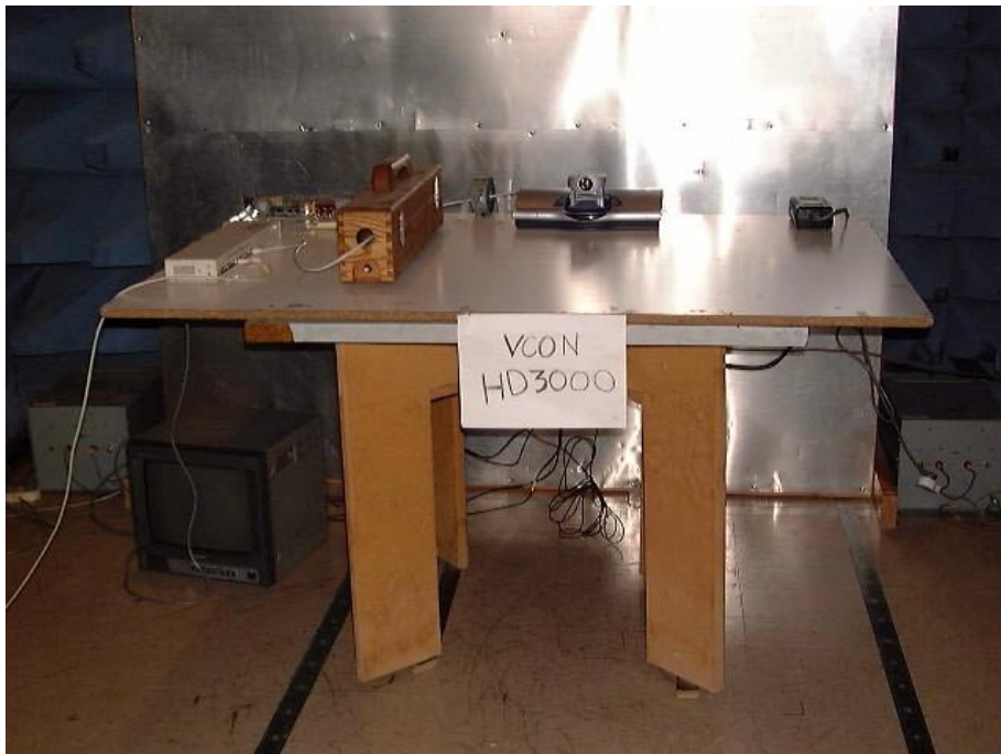
Figure 32. Conducted Emission From Telecommunication Lines Test
