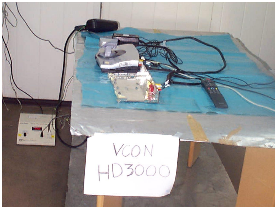
Figure 36. Immunity to Electrostatic Discharge Test
