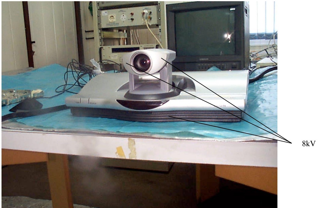
Figure 25. ESD Test Points
